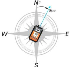
Depending on the compass orientation (sec. 2.2.4), indicated is the orientation of the instrument itself or the plane on which it is installed.
